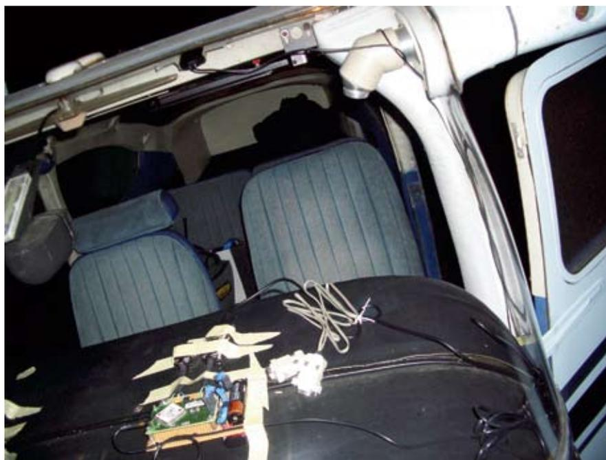
With the antenna mounted at the top of the windshield (upper left in photo), the GPS pseudo-attitude system (visible on dash) was able to receive signals from almost all satellites visible in the sky.
