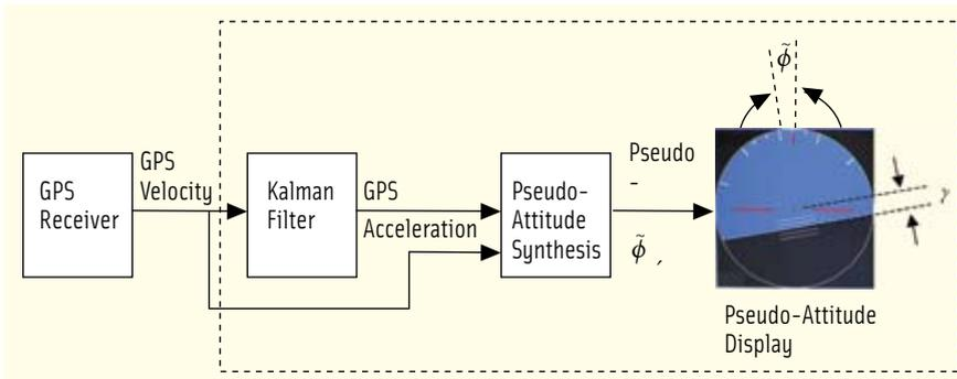
FIGURE 2 Block diagram of pseudo-attitude system
