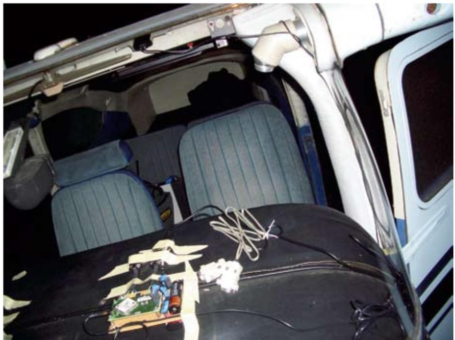
With the antenna mounted at the top of the windscreen (upper left in photo), the GPS pseudo-attitude system (visible on dash) was able to receive signals from almost all satellites visible in the sky.
